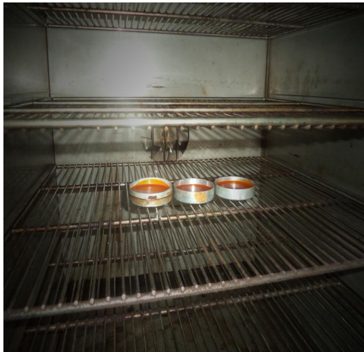
Figure 3. Dishes containing palm oil samples in the oven during moisture content determination.
